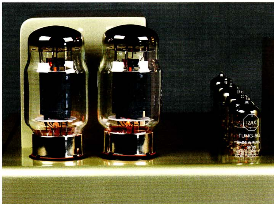
RIGHT: Aside from some solid-state circuitry in the phono section, for quietness, this baby is all-tube: maintaining its purity, the new Quad uses four KT66s, fed by four ECC88s and two ECC83s
